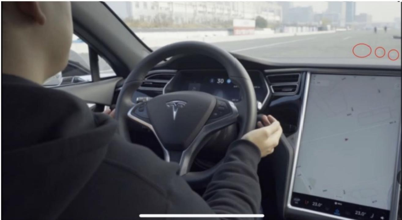
In-car perspective when testing, the red circle marks, the interference markings are marked with red circles
