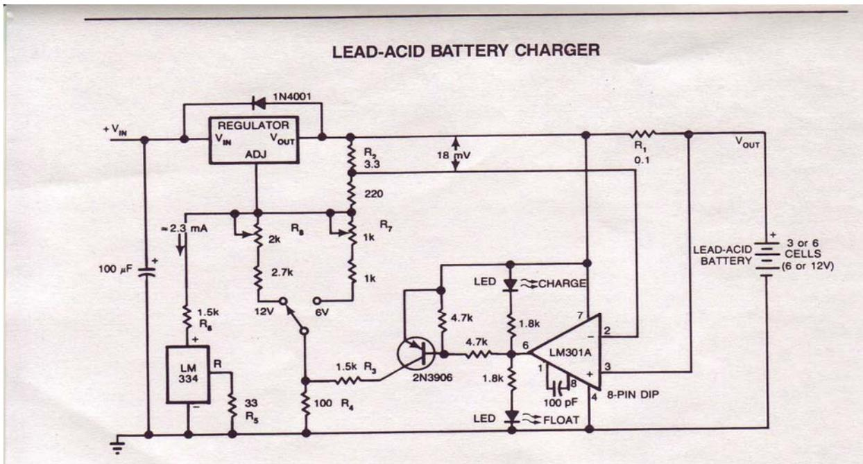
Figure 8: Lead-Acid Battery Charger Circuit Diagram
