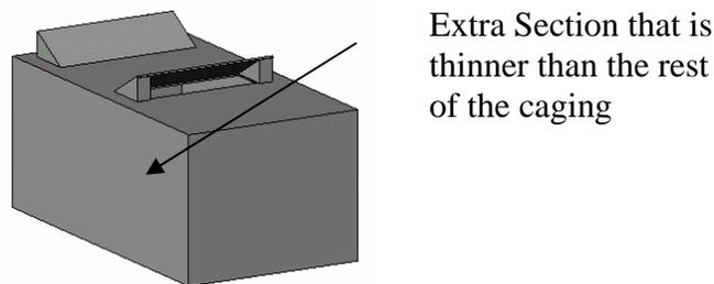
Figure 4: Cage designed for sliding fit
