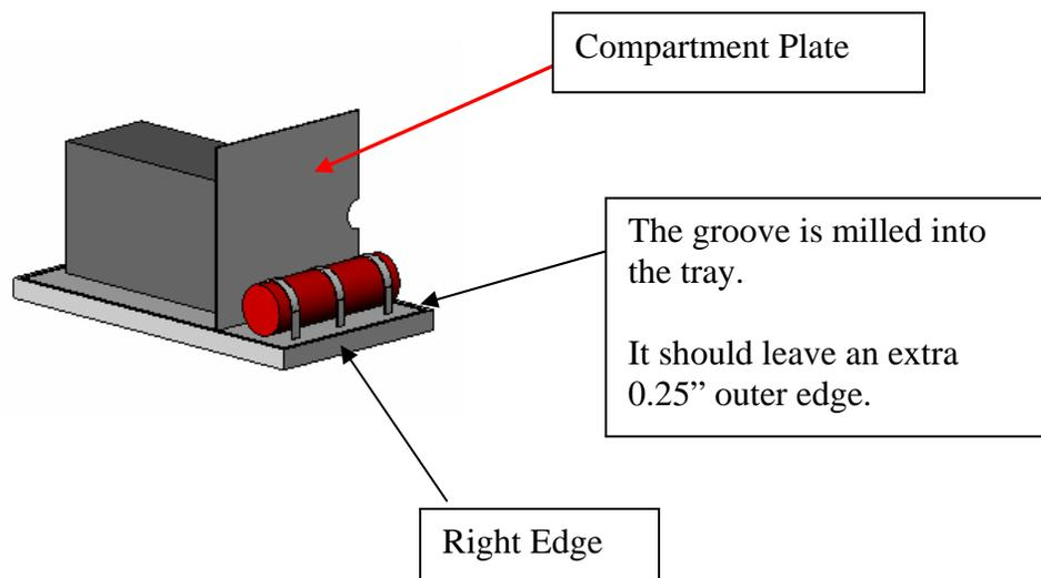
**Step 3: Welding the compartment plate to the tray**
