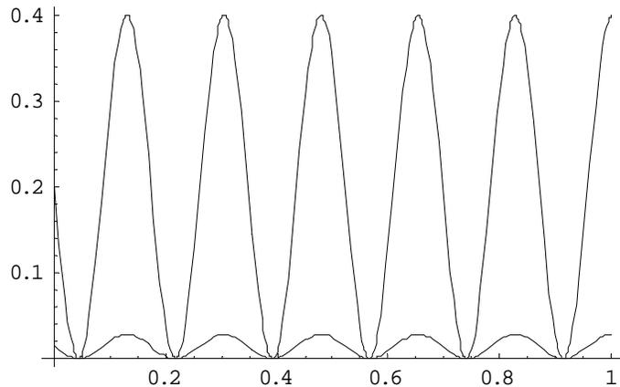
The above graph shows that the ASTM standards require a much higher displacement of the stack than the standards of the stack specify. However, this is a very preliminary vibration analysis. It does not account for the fact that the stack can withstand a constant acceleration of 5g from 60Hz to 150Hz, which is much higher than the 7 Hz vibrations that the ASTM standards specify.
