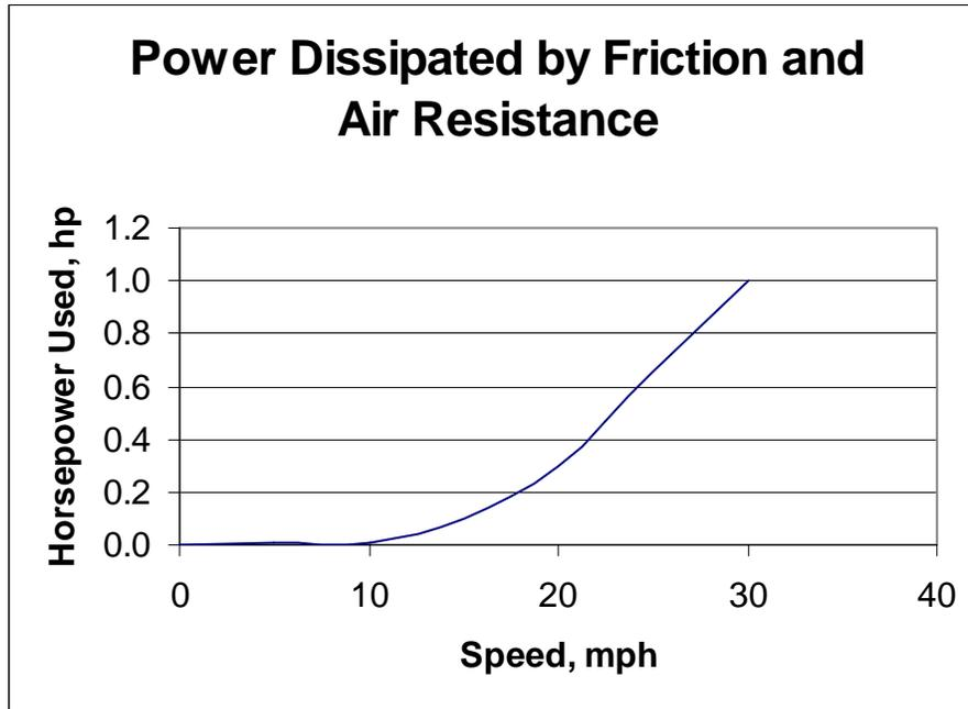
**Figure C.1: Power dissipated by friction and air resistance.**
